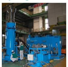
This system allows the pressure in the tank to pressurize and decrease repeatedly in the maximum condition that is 140MPa and 40s/cycle by water. Rapture test of tank by pressurization up to 380 MPa can be carried out.
