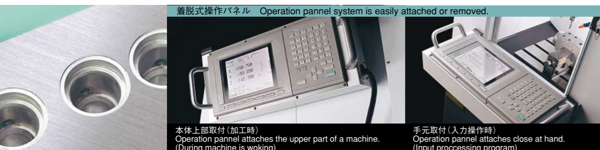
着脱式操作パネル Operation panel system is easily attached or removed.
