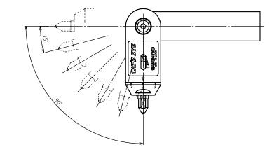
$<sup>^*\,{\</sup>rm Tool}$  angle can be adjustable in the range of  $\pm$  90  $^\circ~\,$  in. 15  $^\circ~\,.$
