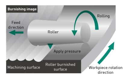
Smooth out uneven machined surface by rollers.
